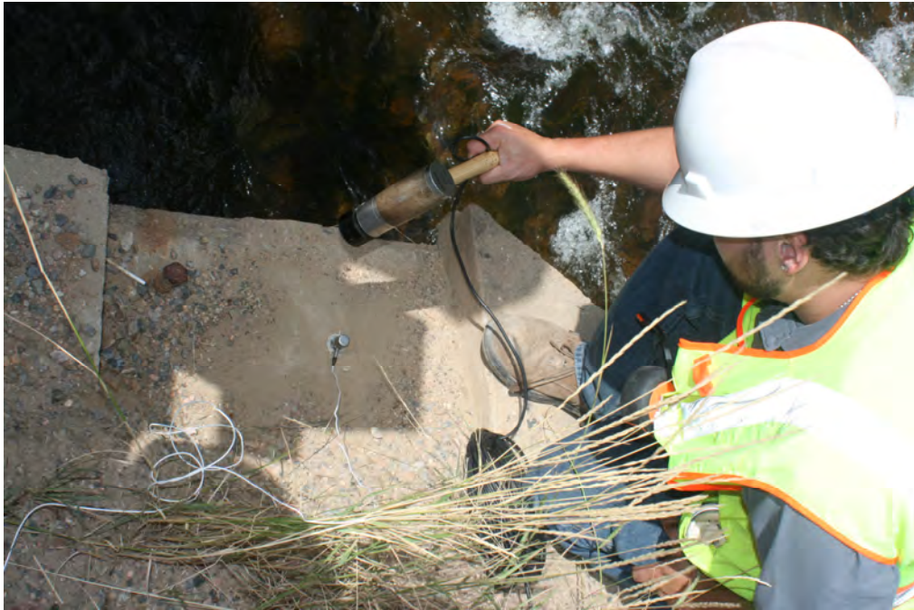
Figure 1 – SE/IR Testing from the top of the East foundation wall.
